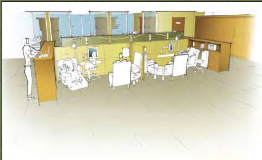
Figure 3. These Infusion Cubes are designed with two zones—one to provide nurses easy access to the patient, and the other for family to sit with their loved one comfortably without being in the way. The nurses have storage and work surfaces to complete drug preparation and do charting at the point of care.
